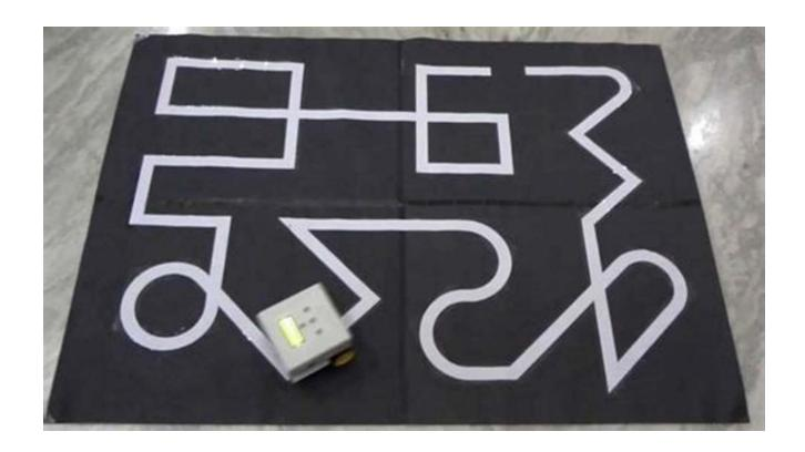
The Line-Following Robot is an excellent project for beginners in robotics. This design focuses on developing a robot that can follow a line using optical sensors. By calibrating the sensors and programming the robot's movements, you will train it to stay on track. It's a great way to understand the basics of programming and sensor integration.
